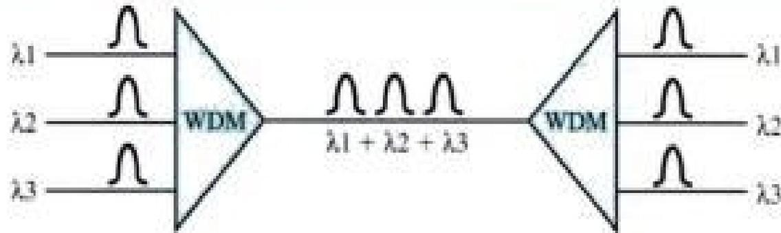
Very narrow bands of light from different sources are combined to make a wider band of light. At the receiver, the signals are separated by the demultiplexer.
