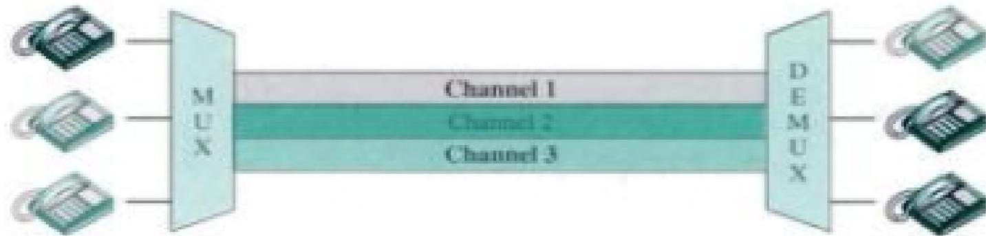
Transmission path is divided into three parts, each representing a channel to carry one transmission.
